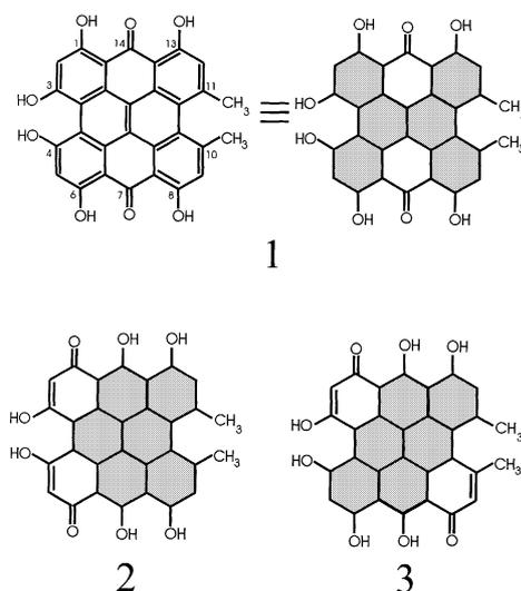
**Fig. 1.** Three tautomers of hypericin; in the text **1**, **2** and **3** are denoted by  $Q(7, 14)$ ,  $Q(1, 6)$ , and  $Q(1, 8)$ , respectively; the conjugated benzenoid domains in these molecules are indicated by shading
